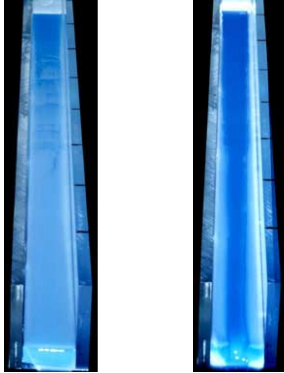
Fig. 3: Views up the channel towards the source, showing the formation and meltback of a chill layer in a thermal erosion experiment. The first photograph (left) was taken after 2 minutes, and shows the white chill layer that has formed on top of the original cold ground (dyed blue). The second photograph (right) was taken after 36 minutes, and shows that the chill layer has been completely eroded along the centre of the channel but still remains along its sides.
