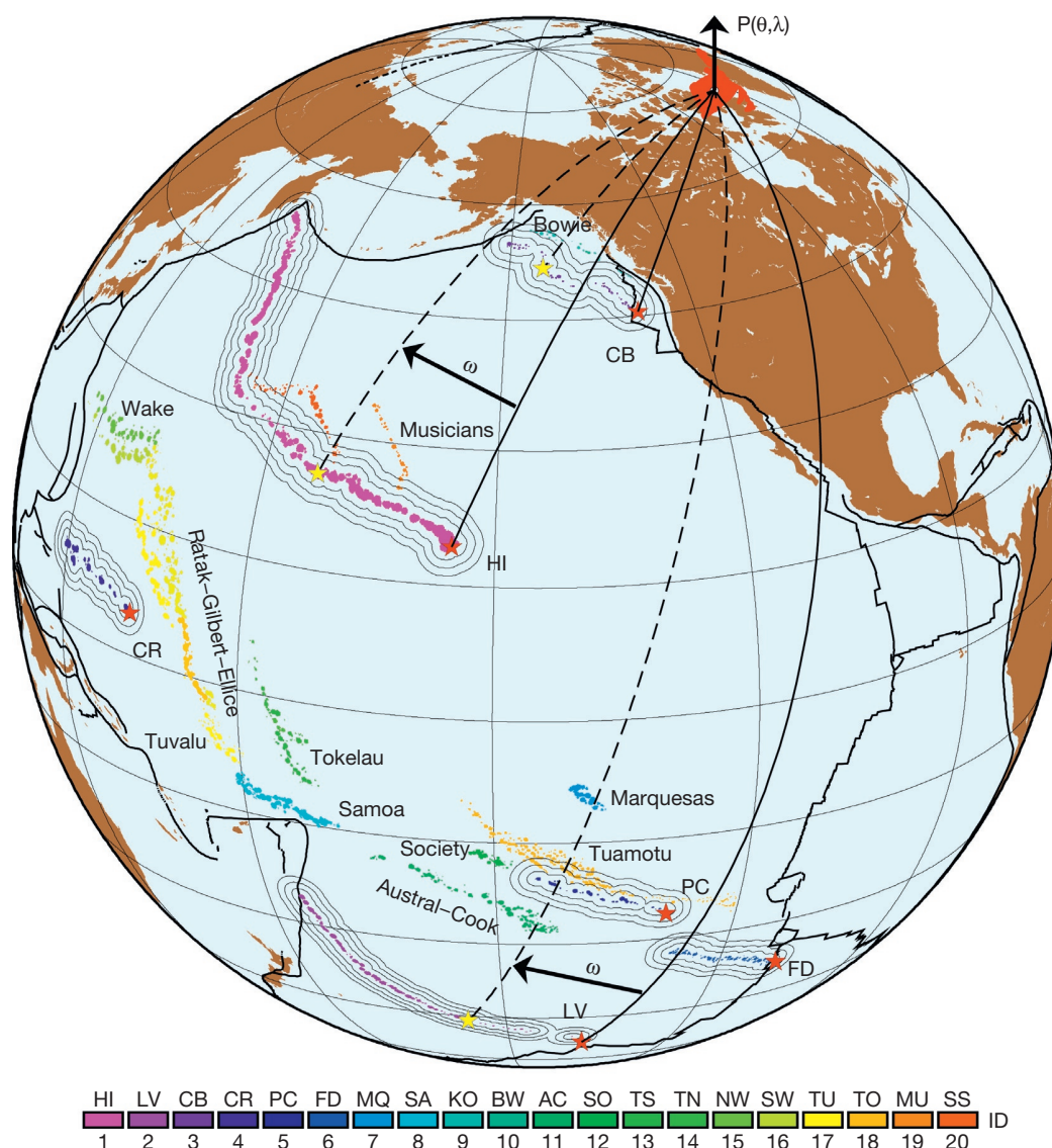
Figure 25 Seamount data constraints generated from the Wessel and Lyons (1997) seamount database. Unique chain ID numbers have been assigned to each seamount (as color-coded). The PFRM works by brute-force grid search of all possible rotations. For each trial rotation, here exemplified by the rotation pole P at (70^\circ \text{ N}, 66^\circ \text{ W}) with an opening angle of \omega = 18^\circ , the M hot spot locations (red stars: HI, Hawaii; LV, Louisville; FD, Foundation; PC, Pitcairn; CR, Caroline; and CB, Cobb) are reconstructed (yellow stars). If two or more of these reconstructed points fall on or very close to their respective seamount chain, the rotation is included in the further analysis. The cluster of poles near P (red dots) represents all the rotations that passed the test for all opening angles in the 17^\circ \leq \omega \leq 19^\circ interval. Additional chains (shown but not used in the modeling) are Marquesas (MQ), Samoa (SA), Kodiak (KO), Bowie (BW), Austral-Cook (AC), Society Islands (SO), southern (TS) and northern (TN) Tokelau, southern (SW) and northern (NW) Wake, Tuvalu (TU), Tuamotu (TO), Musicians (MU), and Liliuokalani (SS). Figure redrawn from Wessel et al. (2006) .
