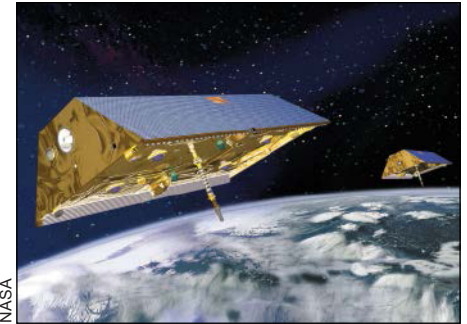
Twin GRACE satellites measure tiny variations in Earth's gravity from accelerations and decelerations along their orbits.
