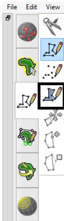
Figure 17. Under the 'Digitisation Tools' icon, you will find Measure, Digitise new Polyline Geometry, Digitise new Multi-Point Geometry, Digitise new Polygon Geometry (circled), Move Vertex, Insert Vertex and Delete Vertex.
