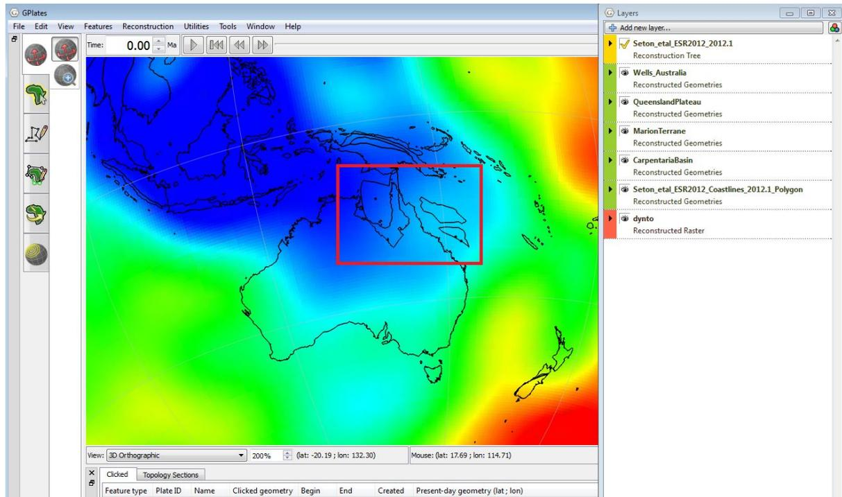
**Figure 10.** View of the Australian region with Gulf of Carpentaria basin outline and the Duyen-1 well (black dot) as well as the Marion and Queensland Plateau polygons and other well data. Background are time-dependent dynamic topography images.
