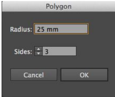
Figure 6. Choosing the size and number of sides of a newly created Polygon (triangle).
