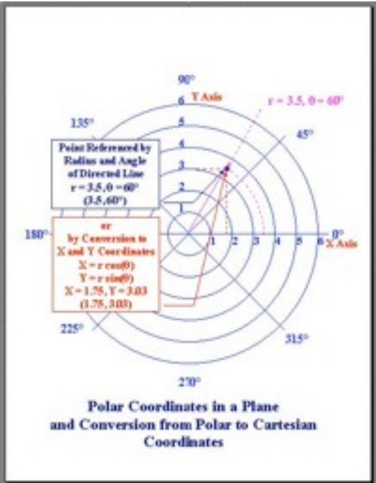
Figure 4.4: Polar coordinates in a plane and conversion from Polar to Cartesian Coordinates.
