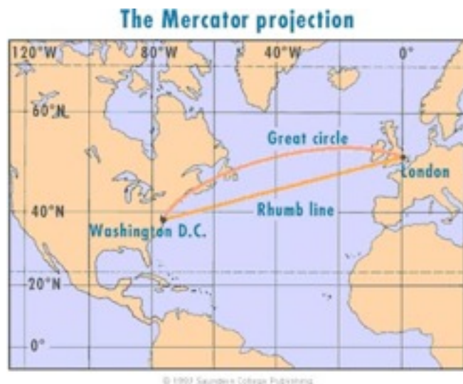
Figure 5.15: Mercator projection showing the difference between the rhumb line and the great circle between Washington D.C. and London. The great circle represents the shortest distance however, the rhumb line is more useful for navigation as it represents a line of constant bearing. A navigator wanting to travel from London to Washington D.C. need only draw a straight line on a Mercator map, measure the angle and determine the bearing to take.
